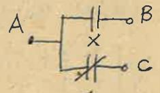
Same relay coil controls both of the contacts.
