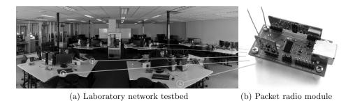
Fig. 2. Monash WSRNLab's [14] experimental wireless mesh network.
