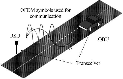
Figure 1. Parts of a WAVE system
