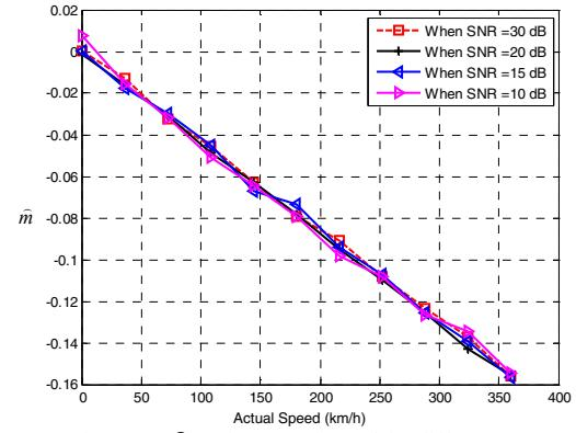
Figure 6.  $\hat{m}$  against actual speed for different SNRs
