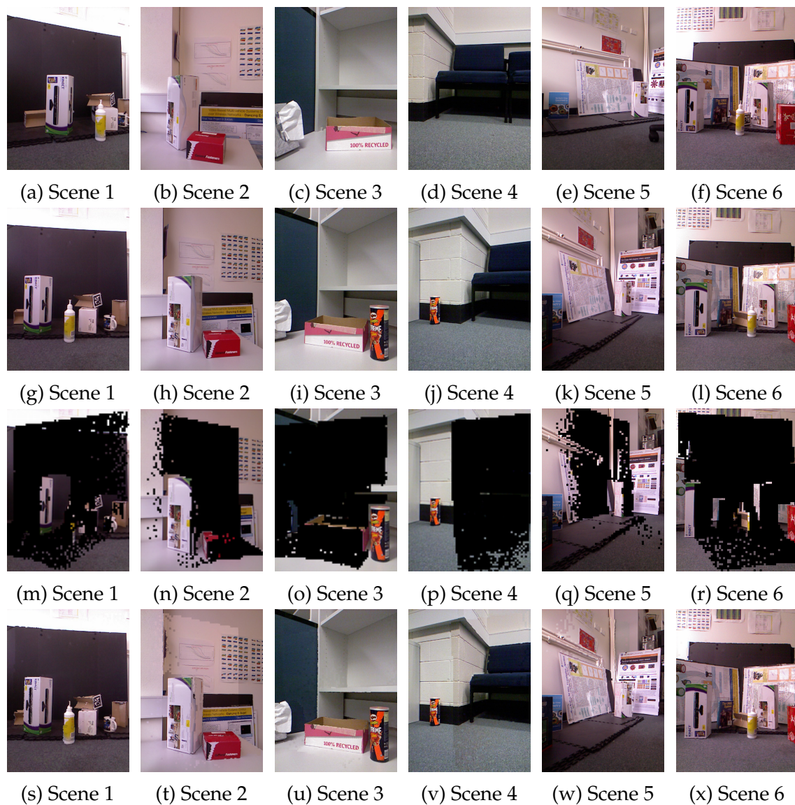
Figure 5.11: A demonstration of the scheme over six sets of images captured by the RGB-D sensors: First and second rows show the images captured by Sensors a , and b respectively. In the third row, image blocks transmitted by Sensor b are shown (here black regions denote the image blocks that are not transmitted). The fourth row shows the reconstructed images at the receiver side using the data sent by Sensor b .
